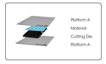
Important: When using AccuQuilt Go dies or Sizzix cutting dies, do not have fabric hang over the dies, it may jam the machine.
