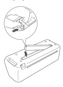
Dampen a soft lint-free cloth with water and firmly wring it out, and then wipe the scanner glass at the inside on the bottom of the machine.
