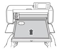
► The mat is fed in, and the "Start/Stop" button in the operation panel lights up.
