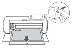
Peel off the material from an area that is easily removable, such as a corner, and then slowly peel while maintaining an even pressure.
