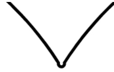
Offset is too high: Divots appear inside and around corners
