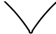
Offset is too high: Divots will appear around corners
