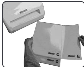
Optional: Place the shim(s) between base platforms ('B', 'C', or 'D')
